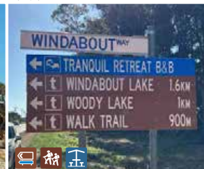
Fisheries Rd/Windabout Way intersection - Too much information, this intersection should have a double sided brown directional sign "Woody Lake Reserve" and the appropriate AS symbols. B&B sign should be below.
