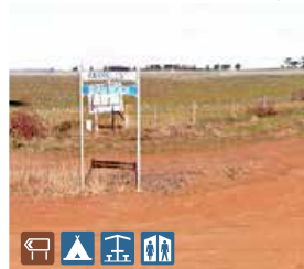
South Coast Hwy/Farrells Rd intersection currently is poorly signed. This intersection should have a double sided brown directional sign with sign with AS symbols for camping, picnic shelters and toilets.
