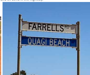
South Coast Hwy/Farrells Rd intersection currently is poorly signed. This intersection should have a double sided brown directional sign with sign with AS symbols for camping, picnic shelters and toilets.
