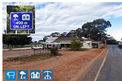
Salmon Gums Rest Area - This rest area has well placed advance warning signs but poorly placed directional signs at the rest area.
