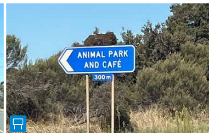
This sign should be an advance warning sign, not a directional sign.
