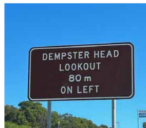
Advance warning signs should be positioned at least 200m prior to the turn-off for vehicles traveling 70kph.
