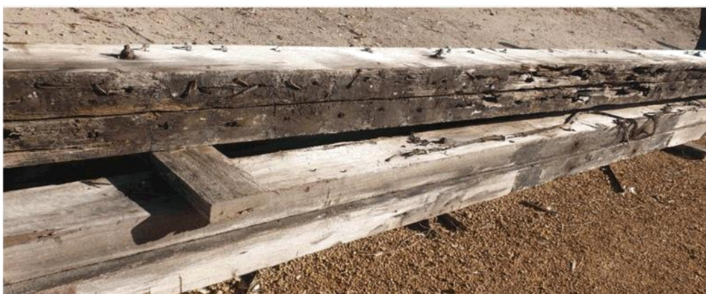
Attached: Photo of borderline Grade 3 (agreed by committee) Jetty timber in top yard of Esperance Men in Sheds Inc.
